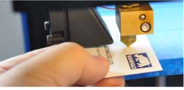
8. Adjust the rest 2 nuts and ensure name card can go through
