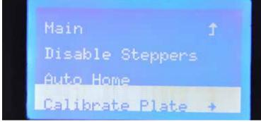
5. Push the button and adjust nut below the plate
